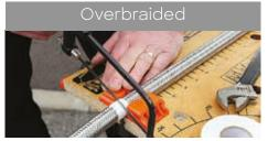
Cutting of overbraided conduit is made much easier by tightly wrapping self adhesive tape around the conduit and sawing through the middle of the tape. The tape should be removed after cutting if EMC screening is required. Ensure you make a straight vertical cut.
