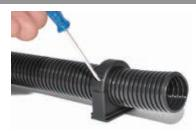
To remove the conduit insert a small screwdriver where it states OPEN. Push down and lever to release. The hinge should then be free to open.
