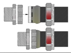
5. Tighten up the nut onto the body with appropriate spanners and to the torque shown on the table.
